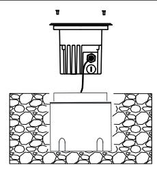
Connect the fitting to the AC power cable and position it into the PVC box. Lock the screws to secure the item's position
