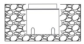
Fix the pvc box into the floor / concrete.
