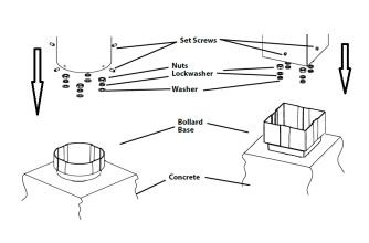
3. Set up the AC connection, Lock the screws and fix the bollard.
