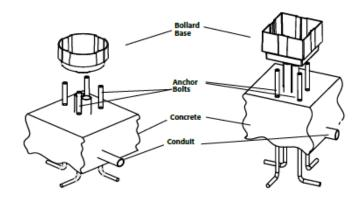
2. Based on your base mounting holes, place the anchor bolts into the concrete with the rigth position / distancing.
