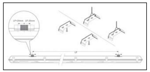
1. Isolate mains power near location so as not to cause electrical hazard. Select desired location to mount LED Weatherproof Batten. Measure and mount included mounting clips to the desired surface.
