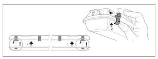
3. Position the diffuser and secure using the clips provided.
