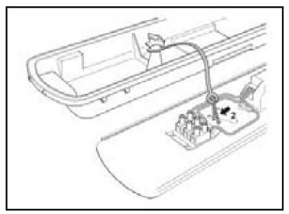
2. Open luminaire by releasing the clips holding the diffuser and remove gear-tray ensuring lanyard is still connected between gear tray and luminaire body. Connect the driver input wires with the main AC.
