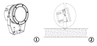
Step①, fix the bracket on the mounting surface by screws. Step②, adjust the bracket as your project needed.
