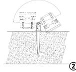
Step  $\bigcirc$ , assemble the spike into the fixture, then insert the spike into ground. (if the fixture received is with the spike, please insert into the ground directly)
