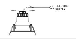
3. press the clips as shown from both sides and put the lamp into the ceiling hole
