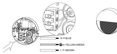
3. Fix the connection ("L""N" into the terminal block).
