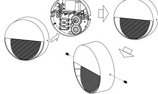
4. Fix the cover with side cap screws.
