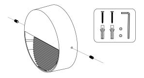
1. Remove the side cap screws with a hex wrench, then open the cover.
