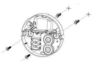
2. Turn off power supply, according to lamp base mounting holes, drill holes in needed position, then fix the lamp base on the wall.
