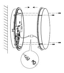
3. Connect the DC plug( if with Emergency , connect the plugs between the battery and driver), put back the cover to the back plate and fix it by screws
