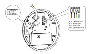
Choose the color temperature with DIP switch if it's the color changeable version (trio CCT), then connect the wires well.
