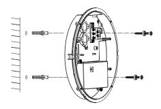
1. Fix the back housing on the wall or ceiling by screws.
