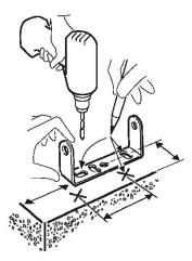
1. Take the suitable size and drill the holes for the installation of the bracket
