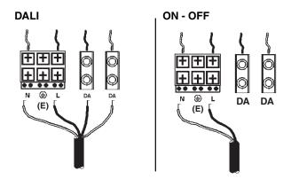
4. Proceed with the wiring connection (always when power is off)
