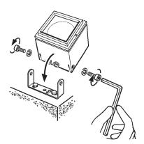
3. Reposition the item onto the bracket and tight the screws accrodignly to the desired item's inclination / position.
