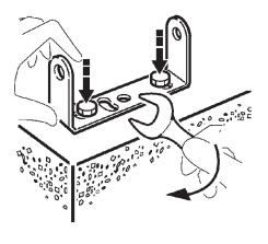
2. Tighten the screws and secure the bracket to the installation surface
