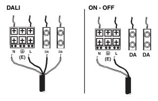
4. Proceed with the wiring connection (always when power is off)
