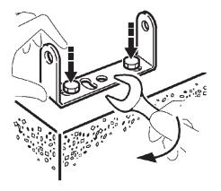
2. Tighten the screws and secure the bracket to the installation surface
