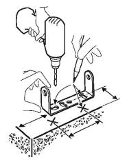
Take the suitable size and drill the holes for the installation of the bracket
