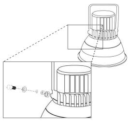
Ensure all fixing screws (bracket) are tight and secure and fix the bracket to the desired surface through the previously perepared holes.
