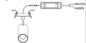
4. press the clips as shown from both sides and put the lamp into the ceiling hole
