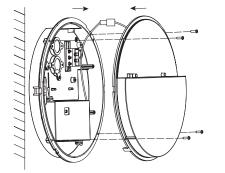
3. Connect the DC plug( if with Emergency , connect the plugs between the battery and driver), put back the cover to the back plate and fix it by screws
