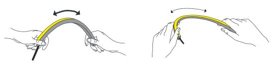
Note. The strip is vertical bendable. Curve the profile only in the indicated axis. In case of non-observance of the given indication, the electrical functionality of the product will be compromised, with consequent luminous interruption of the LED strip. Do not twist it.
