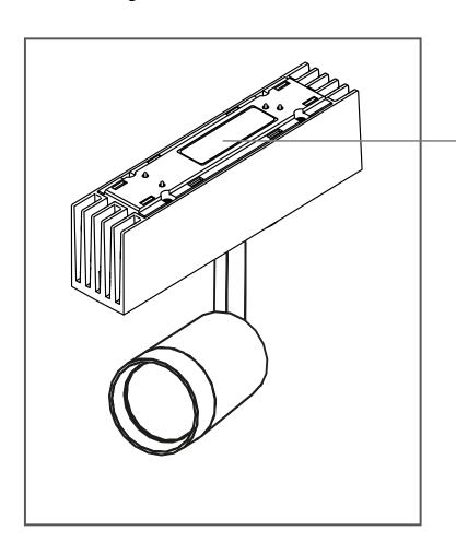
Each Fixture is equipped with a DC/DC converter device carrying the control function.
