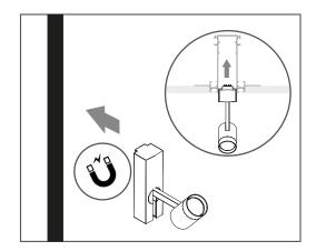
All fixtures of the magnete (magnetic) series works with magnet, so their installation into the profile is very easy: it needs only to position the light as desired and push it up/inside into the track profile till the end.
